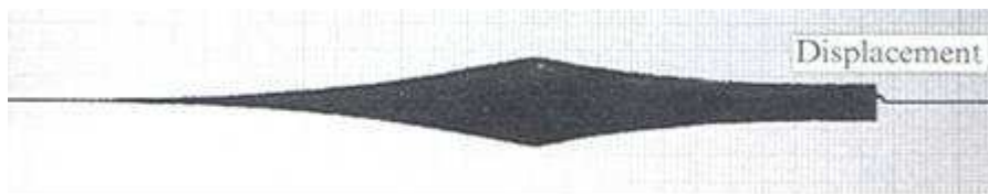
Fig 2.3 Transient response measured at the antinode of an aero elastic model of a conductor after Brika & Laneville (1993)
